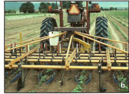
Figure 20. Antennae of precision ag cultivator (A) sense cotton stems and keep cultivator centered on crop row. Spring-hoes uproot weeds and leave cotton unscathed (B).
