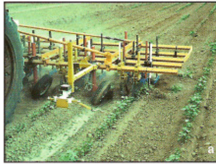
Figure 20. Antennae of precision ag cultivator (A) sense cotton stems and keep cultivator centered on crop row. Spring-hoes uproot weeds and leave cotton unscathed (B).
